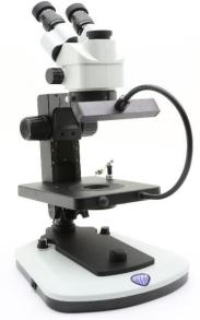
Gemological trinocular stereozoom microscope, 7x...45x, tiltable stand, transmitted & incident light
